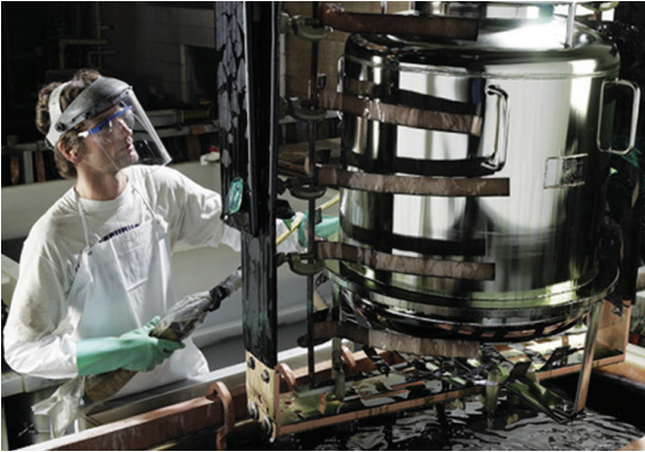
A small / portable vessel emerges from Apache's in-house electropolishing tank.
